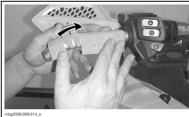
TYPICAL — CORK INSULATOR ALIGNMENT
